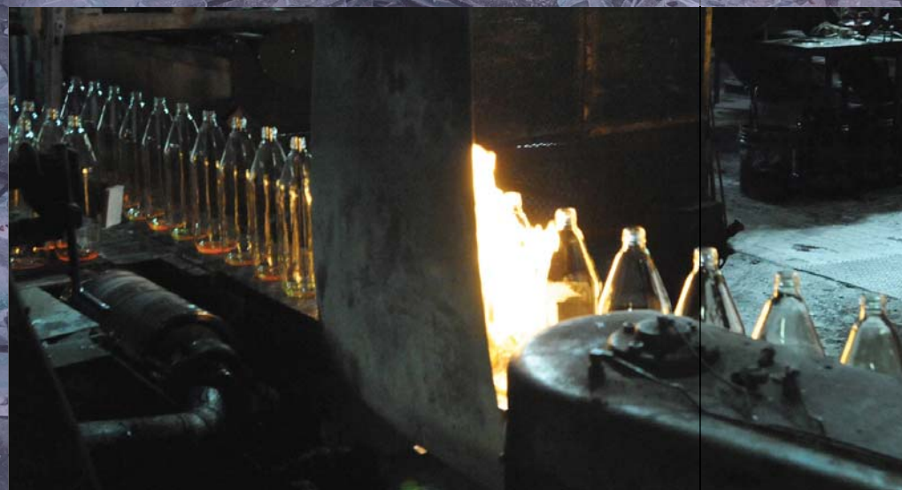
Containers are reheated and gradually cooled to relieve stress in the glass
